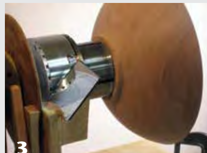
An angled mirror allows for sighting across the top of the vertical piece without having to bend down to the centerline of the spindle for each division line.
