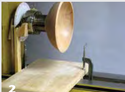
Mount the disk, or polar grid, with the paper facing the tailstock. The author uses a chuck to hold the disk in place, but a faceplate up to 6" in diameter could also be used. The plywood base is clamped to the bed ways.
