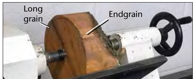
Long grain perpendicular to lathe axis (crossgrain, or faceplate, orientation)
