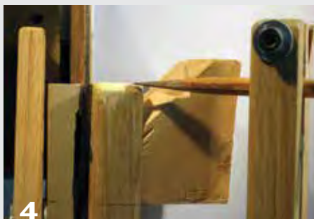
A pencil sharpened with a sanding block to an acute angle improves marking accuracy.
